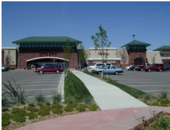
Figure 1119-E: This photograph illustrates how a sidewalk connecting the public sidewalk to the business can be integrated into the required landscaping.
