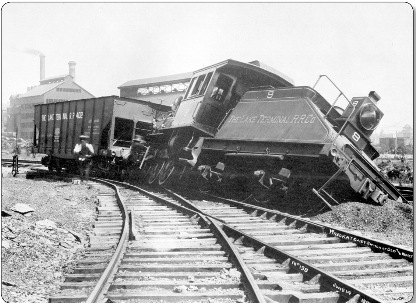
Wreck of Lake Terminal Engine No. 9 and hopper car No. 402, June 14, 1899; engine jumped the track while backing across a switch (Lorain Historical Society).
