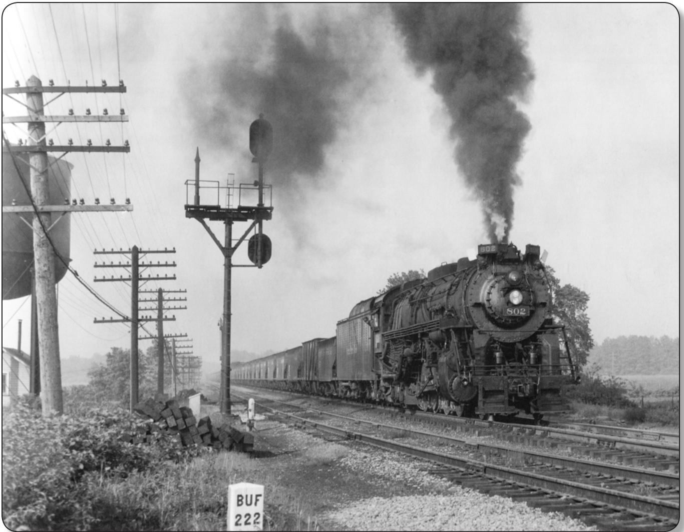
Wheeling & Lake Erie coal train in Lorain County, 222 miles west of Buffalo; Berkshire-type locomotive (2-8-4 wheels), 1955 (J.W. Vigrass).
