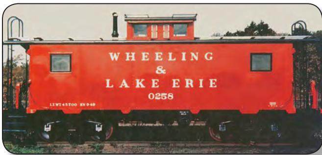
Wheeling & Lake Erie Railway's steel caboosie constructed in 1949. Cabooses were manned rail vehicles coupled at the end of a freight train. They provided shelter for crew, who were required for switching and keeping a lookout for load shifting, any damages, or overheating of axle bearings [a situation called hot boxes]. Cabooses were used on every freight train until the 1980s, when safety laws requiring cabooses and full crews were relaxed (John Corns).
