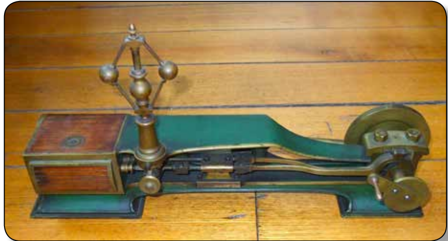
Alexander Rider’s model of his steam engine valve system used to obtain U.S. Patent No. 35,176 in 1861. Rider’s system was used in Capt. John Ericsson’s design of the USS Monitor.
