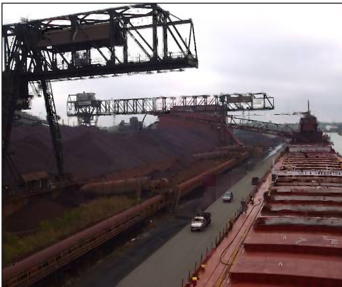
Lee A. Tregurtha unloading iron ore taconite pellets at the Severstal Steel mill on the River Rouge in Dearborn, Michigan.
