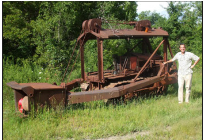
Jim Schilens proudly exhibits his Cletrac tractor Model 40-D, shown here with a Sergeant overhead loader used for mining. This model, built in 1935 and 1936, was power by a Hercules diesel engine.
