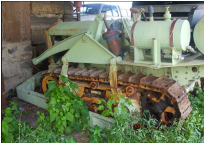
Cletrac tractor Model 55, built from 1932 to 1936, could be fitted with a scraper blade and an air compressor. This model was powered by a Wisconsin gasoline engine.
