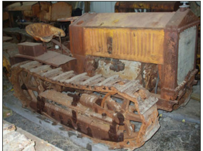
Cletrac tractor Model K-20, built from 1925 to 1928, was a popular model powered by a Wisconsin gasoline engine.
