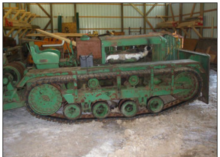
Cletrac tractor Model MG-1, known as the "Bomber Nurse" during World War II, was fitted with rubber tracks for use on sod airfields. This model was built for military applications from 1941 to 1943.
