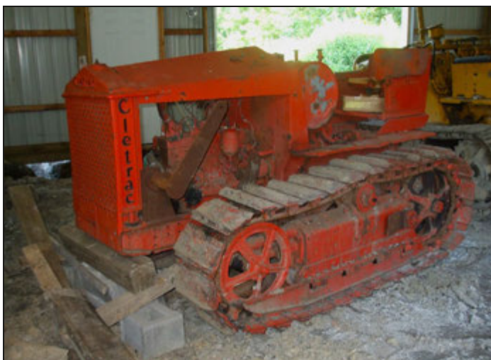
Cletrac tractor Model BG, built from 1937 to 1945, was powered by a Hercules gasoline engine.
