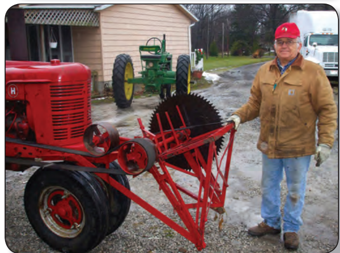
Circa 1954 International Harvester McCormick Farmall H tractor that once belonged to the Burrell family on East River Road at French Creek (upper photo). The Ternes family restored this tractor in 2002. Tim Ternes shows how the belt-driven buzz saw is mounted on the front of Farmall H tractor (lower photo).
