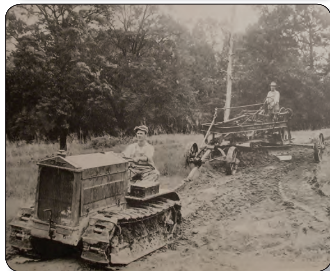
Models K-20 and A-30 Cletrac tractors were successfully used on farms (a) and for road grading (b) in the United States and Europe in the 1920s–1940s (Mike Stockard).
