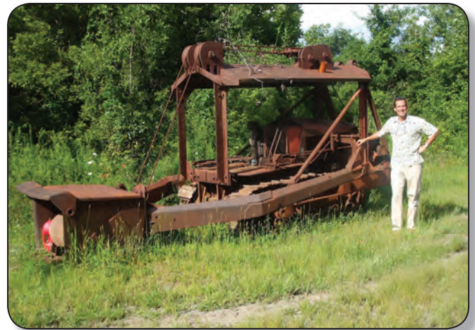
Jim Schilens proudly exhibits his Cletrac tractor Model 40-D, shown here with a Sergeant overhead loader used for mining. This model, built in 1935 and 1936, was powered by a Hercules diesel engine.
