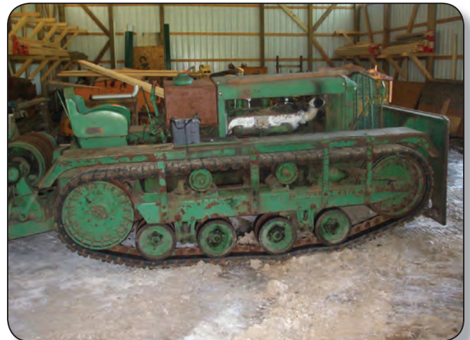
Cletrac tractor Model MG-1, known as the “Bomber Nurse” during World War II, was fitted with rubber tracks for use on sod airfields. This model was built for military applications from 1941 to 1943.
