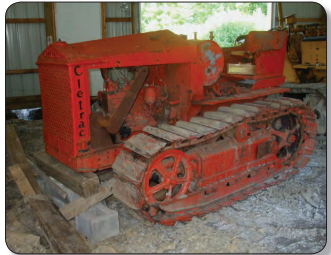
Cletrac tractor Model BG, built from 1937 to 1945, was powered by a Hercules gasoline engine.
