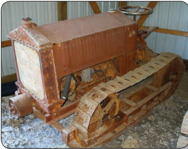
Cletrac tractor Model 12 (W), built from 1919 to 1932, was powered by a Weidley-Cletrac gasoline engine.
