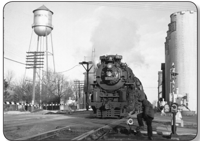
Nickel Plate Road's No. 750 Berkshire-type locomotive (2-8-4 wheel arrangement) at Continental, Ohio, circa 1954 (Don Krofta).
