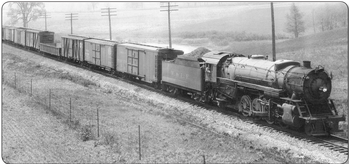
Wheeling & Lake Erie Railway (W&LE) freight train in northeastern Ohio; Mikado-type locomotive (2-8-2 wheel arrangement), circa 1945 (official W&LE photograph).
