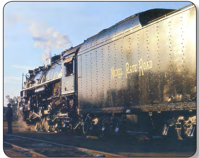
Nickel Plate Road's Berkshire-type locomotive (2-8-4 wheel arrangement) at Conneaut, Ohio, 1968 (Mike Schafer).
