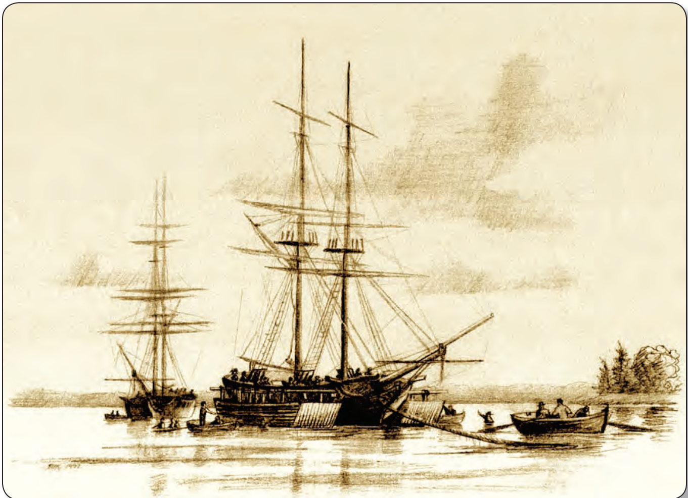
Camel scows used to float the brigs Lawrence and Niagara over the sandbar at Erie Harbor (drawing by Benson Lossing).
