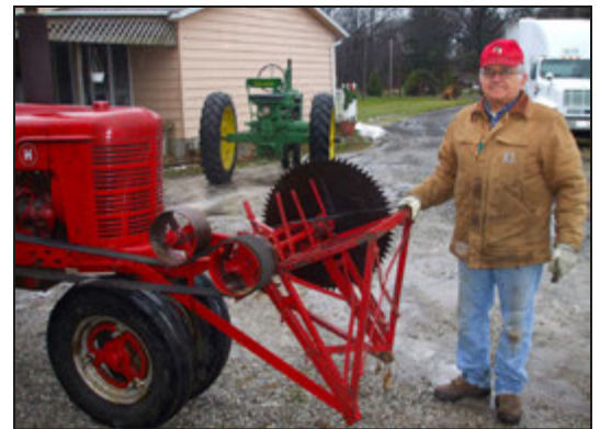
Circa 1954 International Harvester McCormick Farmall H tractor that once belonged to the Burrell family on East River Road at French Creek (left). The Ternes family restored this tractor nearly 10 years ago. Tim Ternes shows how the belt-driven buzz saw is mounted on the front of Farmall H tractor (above).
