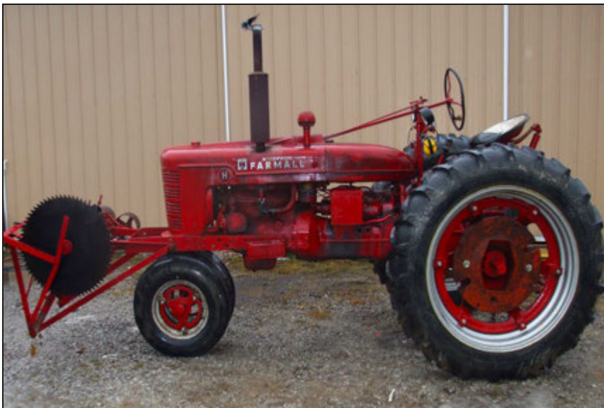
Circa 1954 International Harvester McCormick Farmall H tractor that once belonged to the Burrell family on East River Road at French Creek (left). The Ternes family restored this tractor nearly 10 years ago. Tim Ternes shows how the belt-driven buzz saw is mounted on the front of Farmall H tractor (above).
