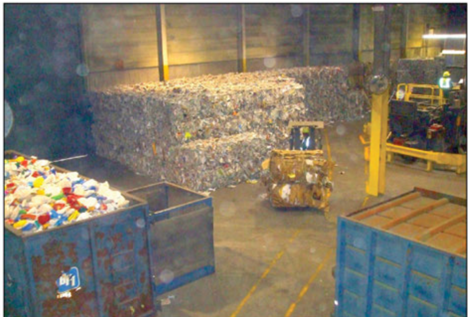
Bales of plastic ready for shipment; Harris baler at upper right; cardboard bale on forklift (center).
