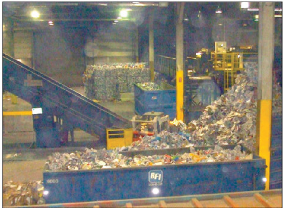
Sorted plastic (right) being loaded on conveyor (left) for transport to baler; bales of aluminum cans in background.
