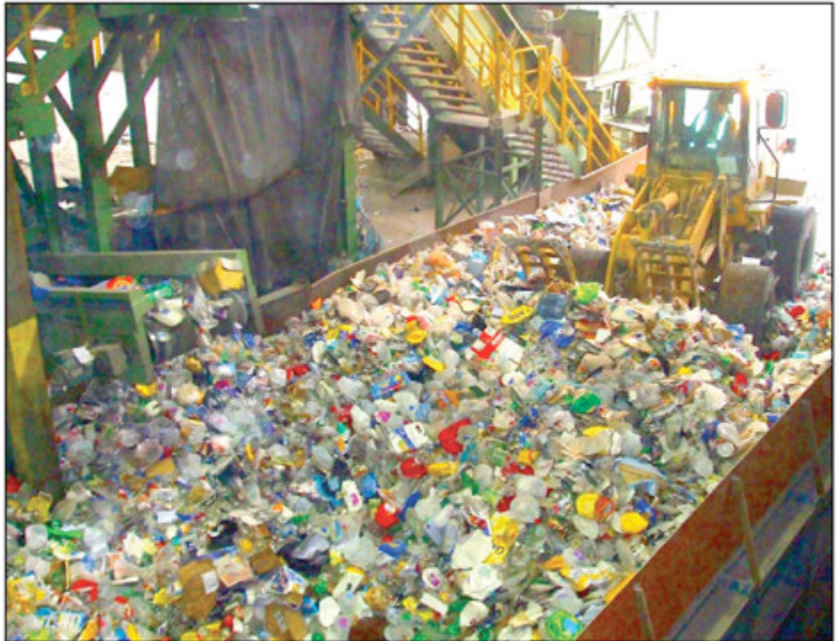
Trash materials being loaded on conveyor to the Star Screens.
