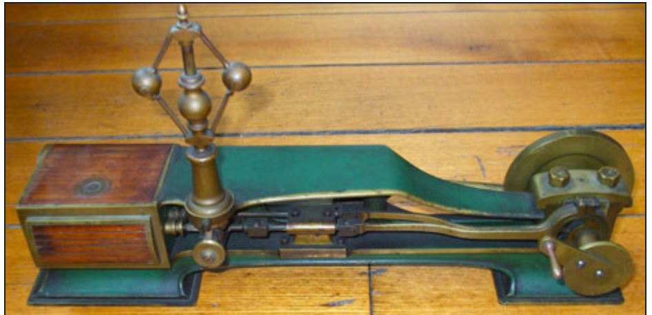
Alexander Rider’s model of his steam engine valve system used to obtain U.S. Patent No. 35,176 in 1861. Rider’s system was used in Capt. John Ericsson’s design of the USS Monitor.
