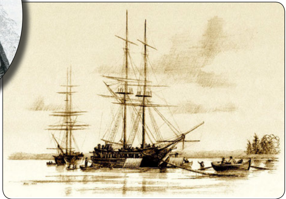
Using camel scows to float the brigs Lawrence and Niagara over the sandbar at Erie Harbor (drawing by Benson Lossing).
