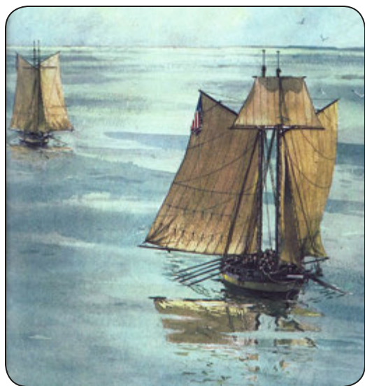
Converted schooners Hamilton and Scourge make their way across a quiet Lake Ontario before a sudden squall sank them in August 1813. Long, heavy oars, known as sweeps, are being used to row the ships under very calm conditions (from a painting by Richard Schlecht).
